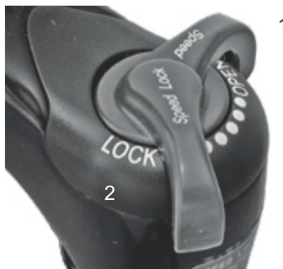
Figure 76: Suntour compression adjuster with the OPEN (1) and LOCK (2) positions
