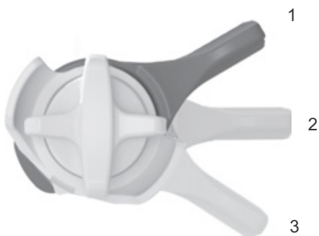
Figure 74: FOX compression adjuster on the rear frame damper with the OPEN (1), MEDIUM (2) and HARD (3) positions
