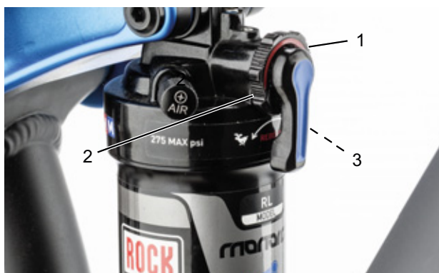
Figure 79: Setting the rebound damper strength on the rear frame damper setting wheel (1)
