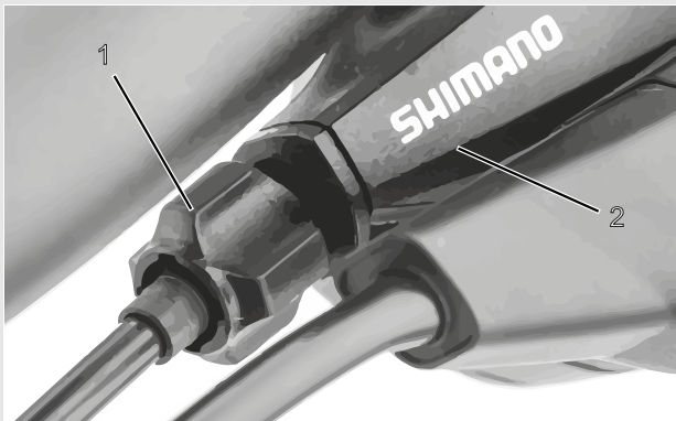
Figure 86: Adjusting sleeve (1) for the single-cable, cable-operated gear shift with shifter housing (2), example
