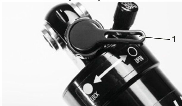
Figure 77: Suntour compression adjuster open (1)
