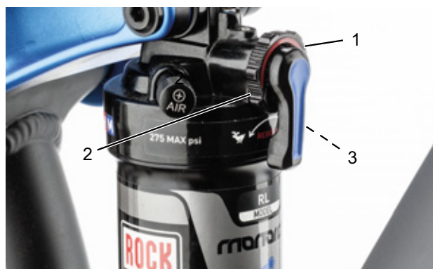
Figure 80: Setting the rebound damper strength on the rear frame damper setting wheel (1)
