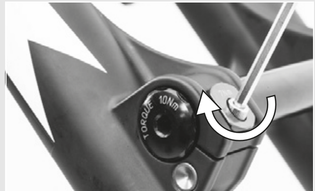
Figure 31: Tightening the axle
