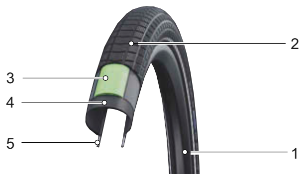
Figure 24: Structure of tube-type tyre
