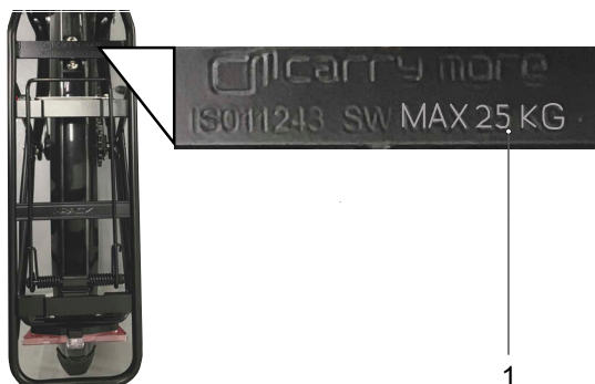
Figure 160: The maximum load bearing (1) capacity is indicated on the pannier rack
