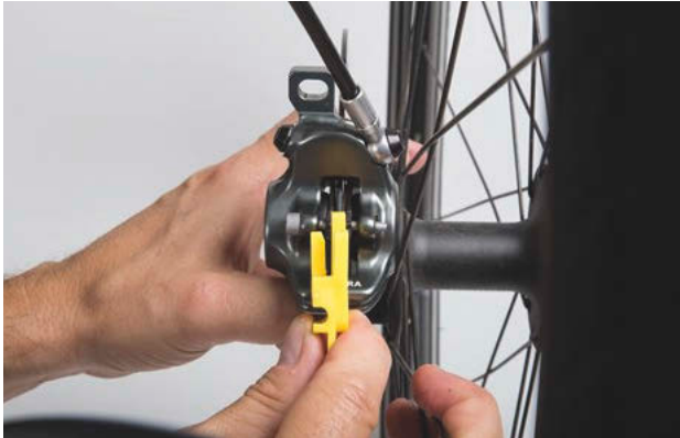
Figure 188: Checking the brake lining when fitted with the help of the transport safety wear gauge
