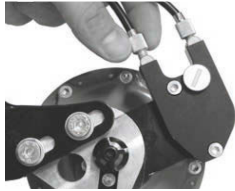
Figure 213: The tension adjuster on ROHLOFF hub versions with external switch control is located on the cable box positioned on the left-hand side
