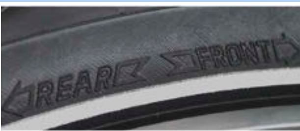
Figure 96: Rotation direction arrow on MTB tyres
