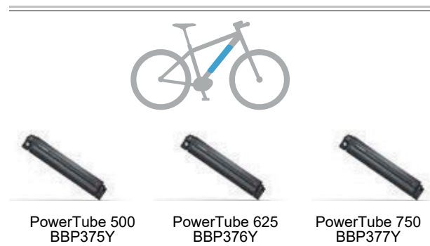
Figure 48: Overview of battery variants
