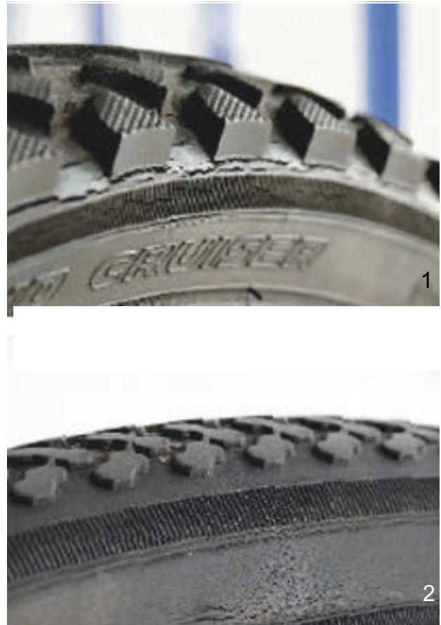
Figure 187: Examples of fatigue cracks (1) and ageing cracks (2)
