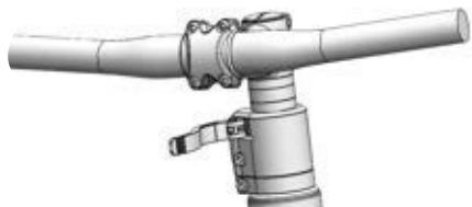
Figure 157: Example of All Up with open stem clamping lever
