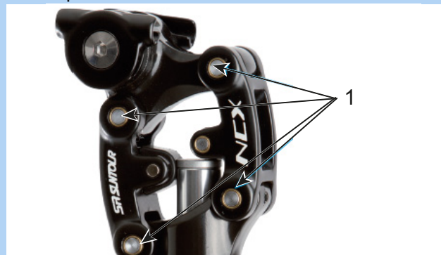
Figure 134: SR Suntour suspension seat post lubrication points
