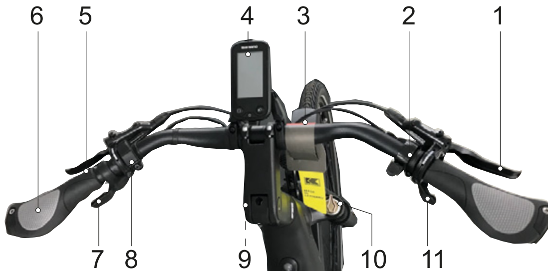
Figure 28: Detailed view of handlebars with SHIMANO SC-E5003 on-board computer, used as example
