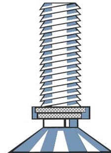
Figura 29: Válvula Schrader
