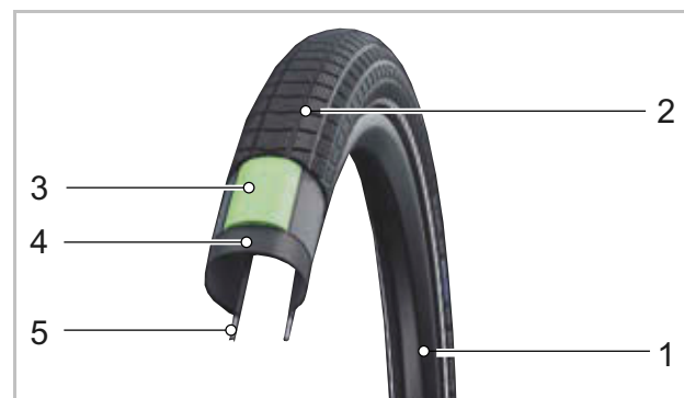
Figure 23: Structure of tube-type tyre
