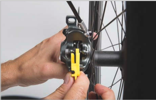
Figure 174: Checking the brake lining when fitted with the help of the transport safety wear gauge
