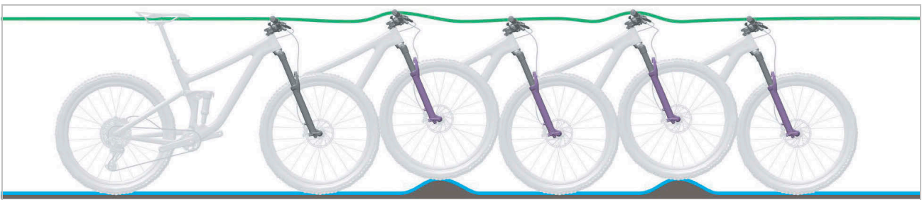
Figure 13: Optimum suspension fork ride performance
