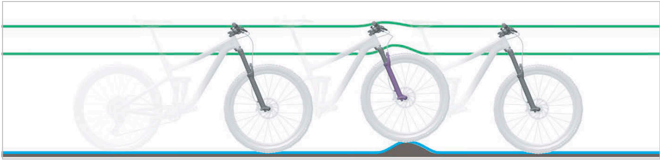
Figure 15: Optimum suspension fork ride performance over bumps
